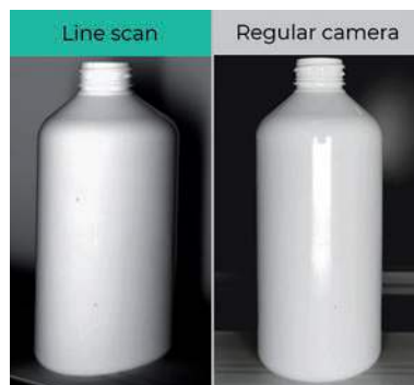
The scan image (left) has no reflections, revealing the upper defect invisible to regular cameras (right)
